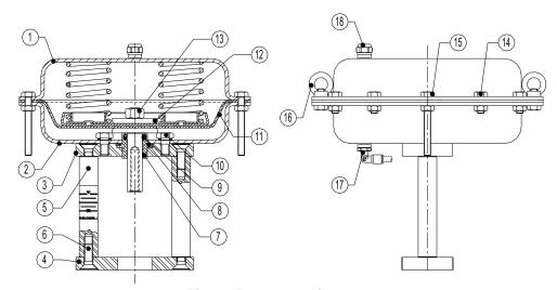
Fig.2 – Reverse action actuator
