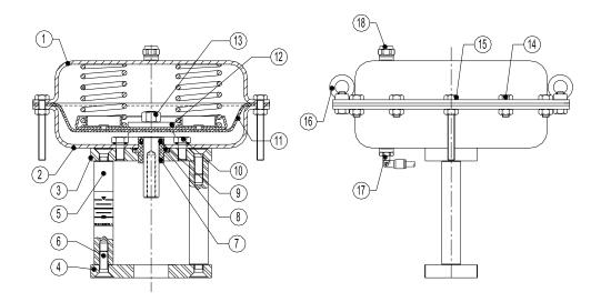
Fig.8 – PA series actuator
