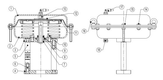
Fig.1 - Direct action actuator
