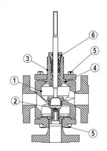
Fig.4 - Replacing the plug
